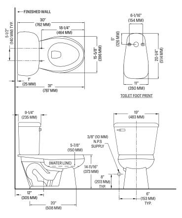
Fixture performance and specifications meet or exceed ASME A112.19.2-2013/CSA B45.1-13 standards, and other state and local codes.
