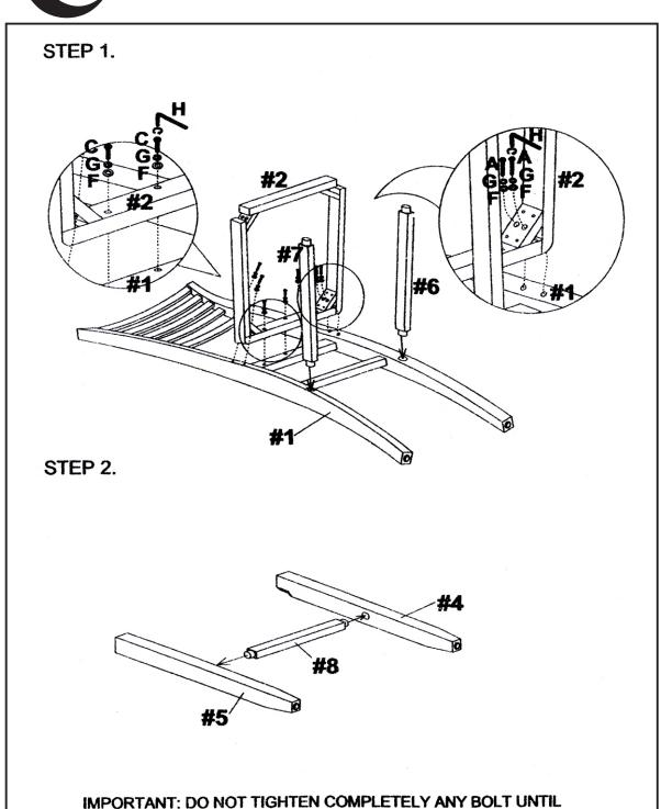
IMPORTANT: DO NOT TIGHTEN COMPLETELY ANY BOLT UNTIL ALL LINED-UP BOLTS ARE CONNECTED TO INSERTED NUTS.
