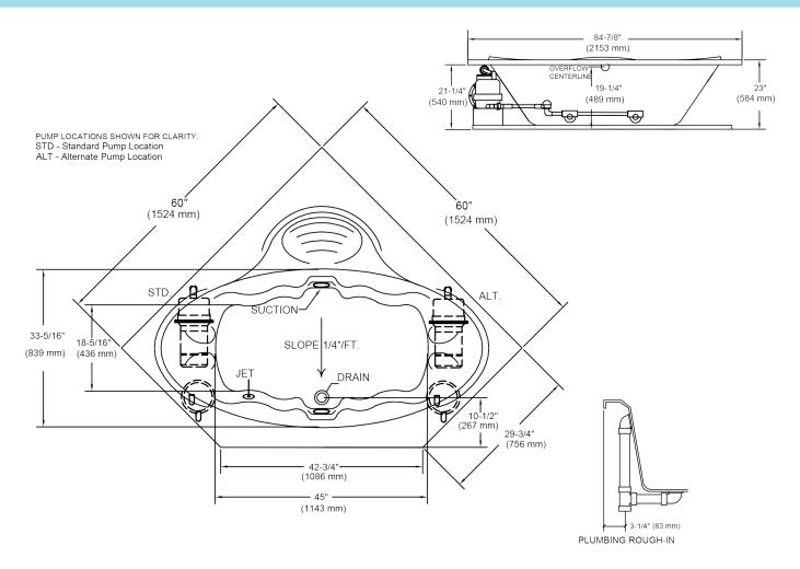
Note: Install this product according to the installation guide. Rough-in measurements may vary 1/4" (=/-).
