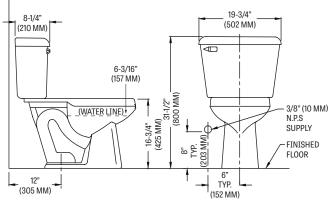
Fixture performance and specifications meet or exceed ASME A112.19.2/CSA B45.1 standards, and other state and local codes.
