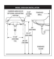
All Mansfield® wall-mount lavatories are supplied with this exclusive one-piece steel hanger. Easily installed and adjusted, it contains 7 holes for solid mounting against wall. Anchoring screw must be used for correct installation. Standard plumbing practice recommends use of both mounting backets and anchoring screws.
