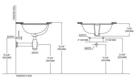
Fixture performance and specifications meet or exceed ASME A112.19.2-2013/CSA B45.1-13 standards, and other state and local codes.
