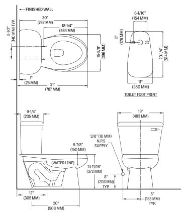
Fixture performance and specifications meet or exceed ASME A112.19.2-2013/CSA B45.1-13 standards, and other state and local codes.
