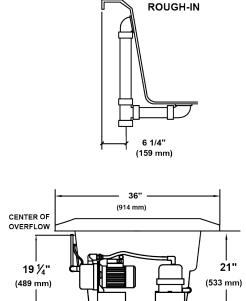
INSTALLER NOTE: DUE TO THE FREEFORM SHAPE OF THIS TUB IT IS RECOMMENDED THAT THE TUB BE ON THE JOBSITE BEFORE MAKING THE FINAL CUT OUT FOR DROP IN INSTALLATION.
