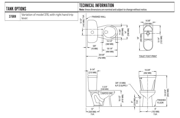
Fixture performance and specifications meet or exceed ASME A112.19.2/CSA B45.1 standards, and other state and local codes.
