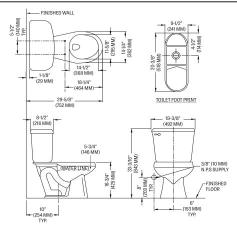
Fixture performance and specifications meet or exceed ASME A112.19.2/CSA B45.1 standards, and other state and local codes.
