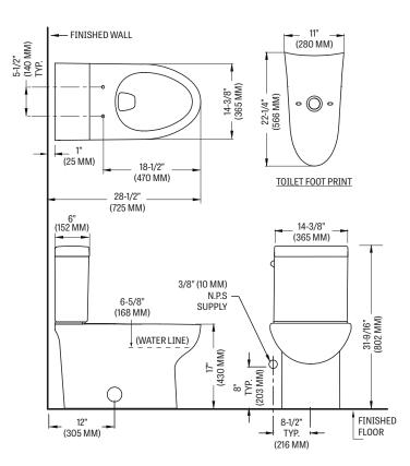
Fixture performance and specifications meet or exceed ASME A112.19.2/CSA B45.1 standards, and other state and local codes.
