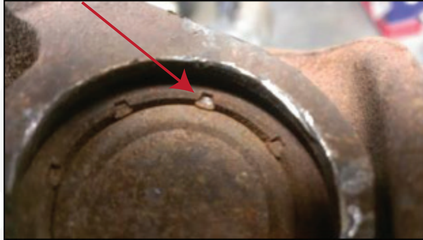
Staked Joint: Notice the dimpled steel to be cut out
