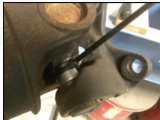
Photos of the sleeve used to press the bearing cap out (with and without zip tie)
