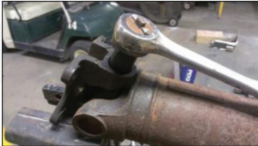
Insert the cutting tool and rotate with socket wrench. USE FORCE
