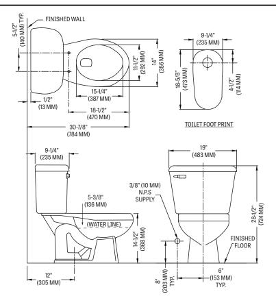
Fixture performance and specifications meet or exceed ASME A112.19.2-2013/CSA B45.1-13 standards, and other state and local codes.
