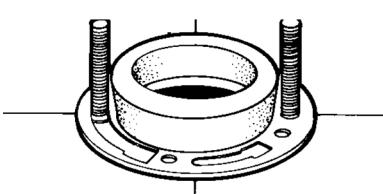
**Alternate way is to place wax ring on the "horn" of the bowl (bowl shown upside down).**
