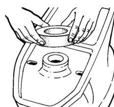
**D****STRADDLE BOWL, LIFT INTO PLACE THEN SET STRAIGHT DOWN ONTO RING AND BOLTS.**
