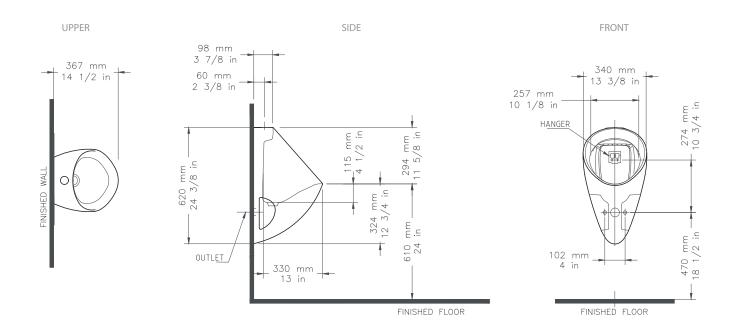
Fixture performance and specifications meet or exceed ASME A112.19.2-2013/CSA B45.1-13 standards, and other state and local codes.
