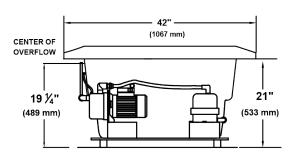
INSTALLER NOTE: DUE TO THE FREEFORM SHAPE OF THIS TUB IT IS RECOMMENDED THAT THE TUB BE ON THE JOBSITE BEFORE MAKING THE FINAL CUT OUT FOR DROP IN INSTALLATION.
