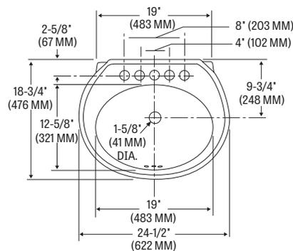
This pedestal lavatory comes with two heavy-duty plastic mounting brackets. Easily installed and adjusted, each contains three holes for solid mounting against wall. Anchoring screws must be used for correct installation. Standard plumbing practice recommends use of both mounting brackets and anchoring screws.
