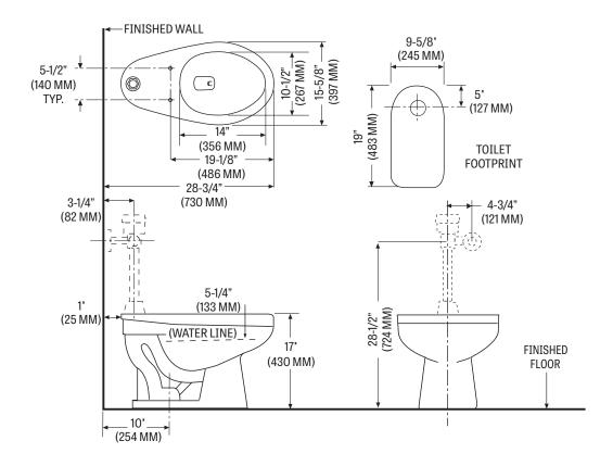
$Fixture\ performance\ and\ specifications\ meet\ or\ exceed\ ASME\ A112.19.2-2013/CSA\ B45.1-13\ standards, and\ other\ state\ and\ local\ codes.$
