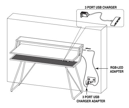
STEP 3 Secure Top (A) to assembly using eight Flat Washers (3) and eight Long Bolts (2). FULLY TIGHTEN ALL LONG BOLTS (2). STEP 4 Connect USB & LED Power Supplies to USB & LED cables on desk.
