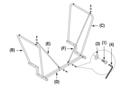
Remove all the parts from carton, separate them into part numbers indicated on the list and make sure part quantities are correct. STEP 1 Attach Left & Right Frames (B & C) to Cross Bar (D) using two Flat Washers (3) and two Short Bolts (1) for each Frame. DO NOT FULLY TIGHTEN BOLTS.
