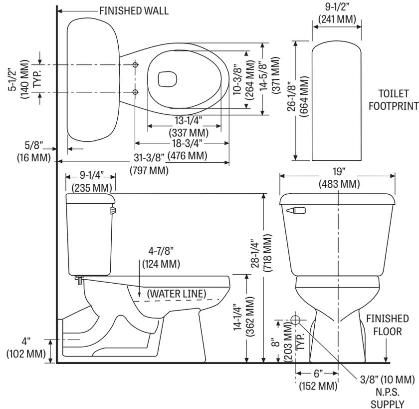
Fixture performance and specifications meet or exceed ASME A112.19.2-2013/CSA B45.1-13 standards, and other state and local codes.
