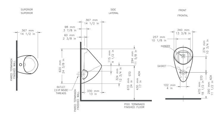
Fixture performance and specifications meet or exceed ASME A112.19.2-2013/CSA B45.1-13 standards, and other state and local codes.
