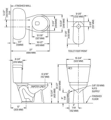
Fixture performance and specifications meet or exceed ASME A112.19.2/CSA B45.1 standards, and other state and local codes.
