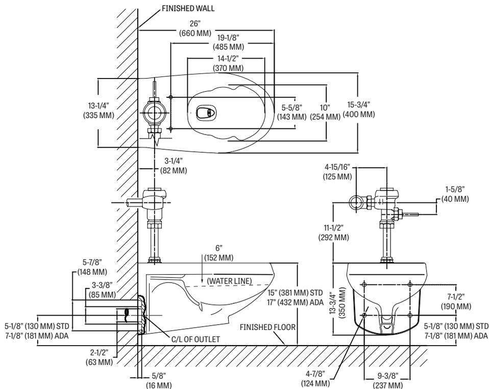
Fixture performance and specifications meet or exceed ASME A112.19.2-2013/CSA B45.1-13 standards, and other state and local codes.
