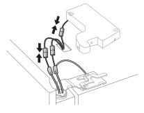
4 Set the hinge cover ④ in place. Insert and tighten the cover screw ⑤.
