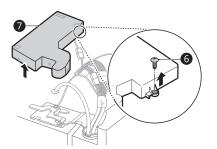
Remove the cover and pull out the tube <sup>(a)</sup>.Disconnect all wire harnesses <sup>(a)</sup>. Unscrew the ground wire <sup>(b)</sup>.
