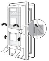
**2** To replace the case, line up the tabs on the case with the slots on the door and push down until it snaps into place.
