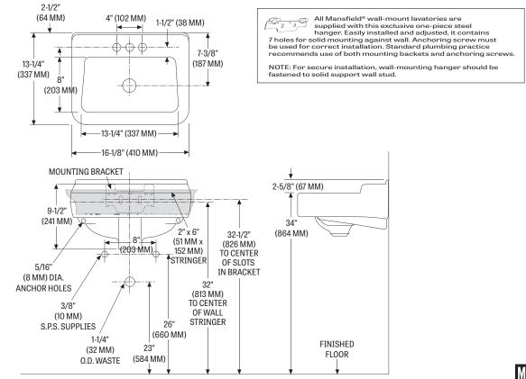
Fixture performance and specifications meet or exceed ASME A112.19.2/CSA B45.1 standards, and other state and local codes.
