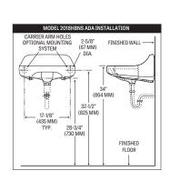
All Mansfield® wall-mount lavatories are supplied with this exclusive one-piece steel hanger. Easily installed and adjusted, it contains 7 holes for solid mounting against wall. Anchoring screw must be used for correct installation. Standard plumbing practice recommends use of both mounting backets and anchoring screws.
